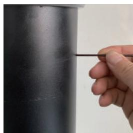
Use the Allen key to press the button from the buttonhole on the pillar.
